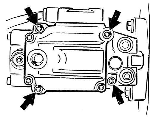
Lift off quantity actuator perpendicularly from pump housing.
